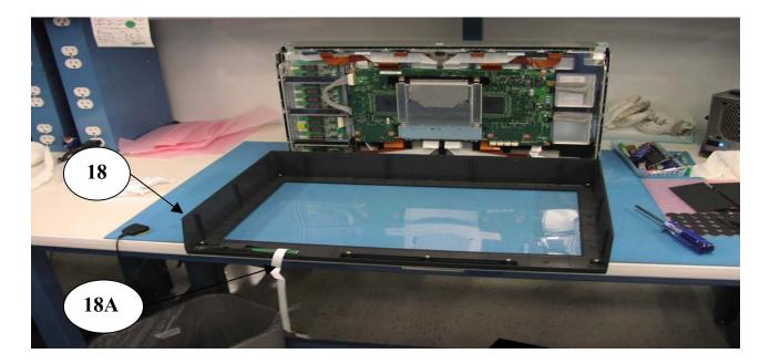
Situate bezel (Item 18) in front of panel. Place the bottom of bezel (with cable- Item 18A) off the table edge to protect the underlying function control buttons.
