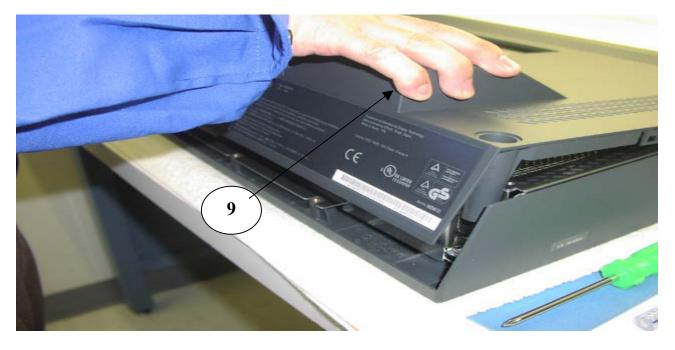
Grasp and unsnap rear housing (Item 9) by lifting until completely separated from monitor.
