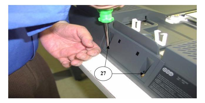
Insert two (2) screws (Item 27) into bottom of monitor.
