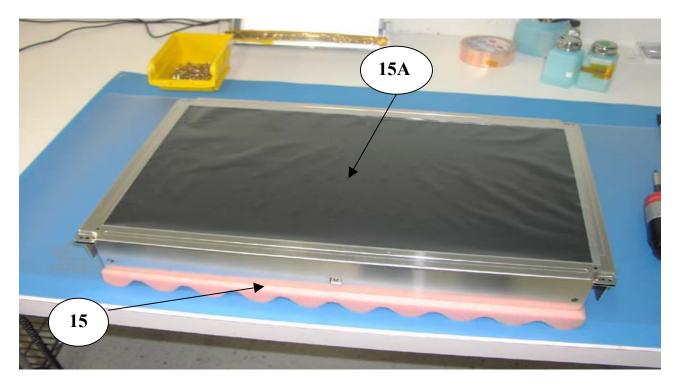
Situate LCD module onto foam cushion (Item 15) to protect underlying PCBs. Install protective mylar film onto front polarizer (Item 15A).
