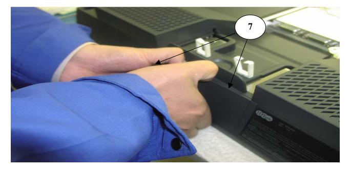
Grasp and unsnap panel (Item 7) that is located on monitor bottom, beneath where base was previously located.
