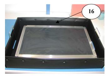
If LCD module (IPN F8991) is to be transported to another work area, use carrier (Item 16). If LCD module is to be disassembled at same work bench, refer to "Assembly (Dis-Assy) Procedure for VIEWSONIC F8991 MODULE" document.
