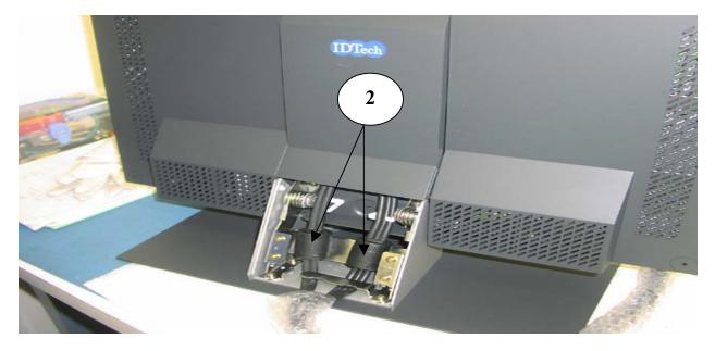
Disengage latch from bottom panel and remove panel to gain access to two (2) cables (Item 2).
