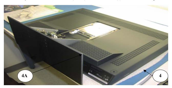
Once both cables are removed from the monitor, lay monitor on bench with screen surface down (protected by foam- Item 4) in preparation for removal of base (Item 4A).
