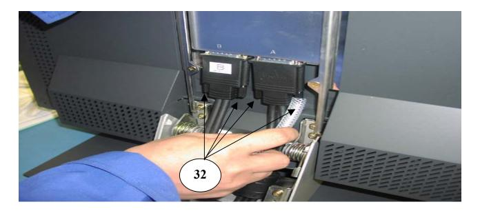
With monitor in upright position, connect two (2) interface cables and secure four (4) screws (Item 32) with the hose tool.
