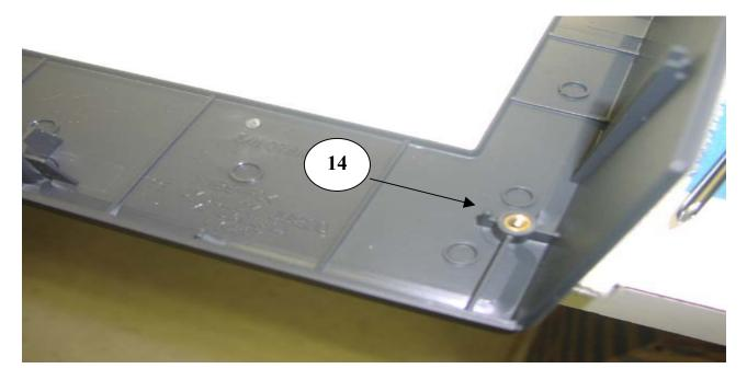
Inspect four (4) guide pins in bezel (one pin in each corner- Item 14) for damage.
