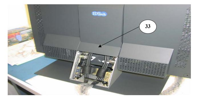
Install upper rear cover panel (Item 33) by snapping into position.
