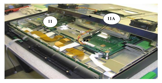
Lift metal backbone (Item 11) and slide toward top of module to enable access to the two (2) fan cables (Item 11A). Disconnect the two cables and note their corresponding mating connectors. Once cables are free, remove metal backbone completely from monitor.
