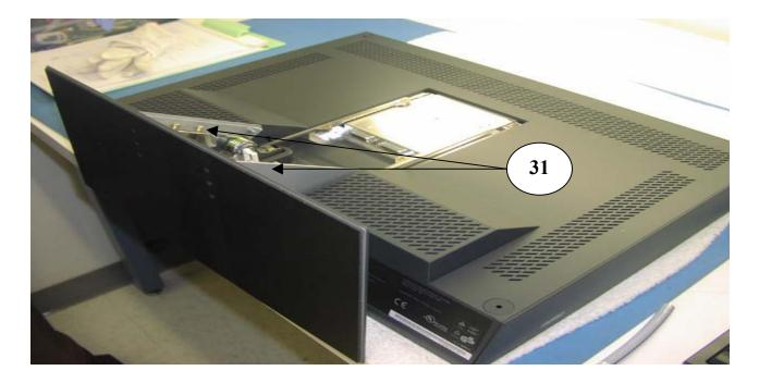
Ensure monitor base (Item 31) is secure before lifting monitor into upright position.
