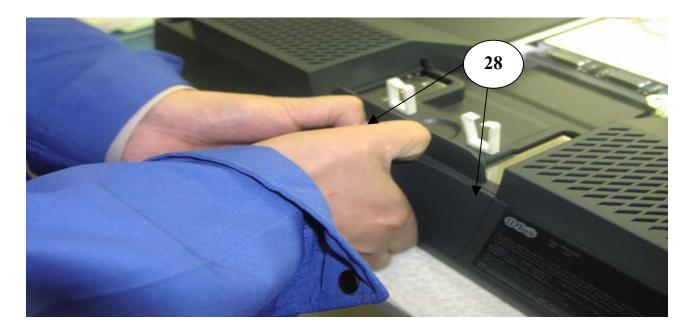
Grasp and install cover panel (Item 28) by snapping into position.
