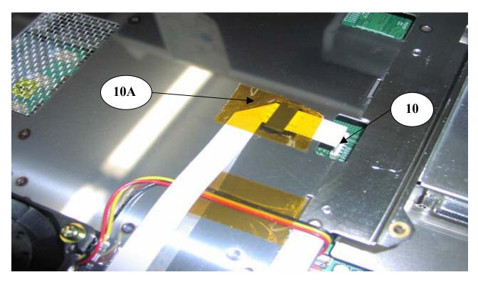
Remove ribbon cable from connector (Item 10). Peel back tape (Item 10A) to disengage cable from metal backbone.
