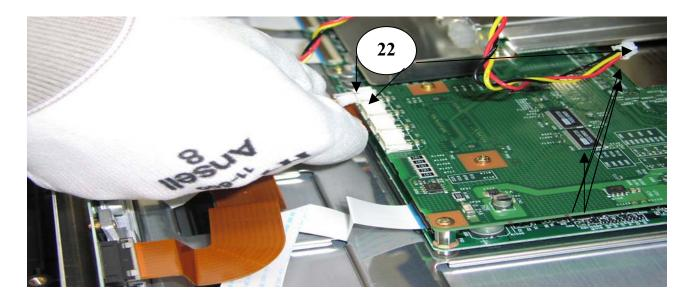
Connect two (2) fan cables into the original connector mates on the PCB (Item 22). Do not mix.
