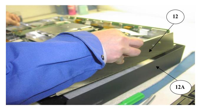
Lift and separate LCD module (Item 12) from monitor bezel (Item 12A).
