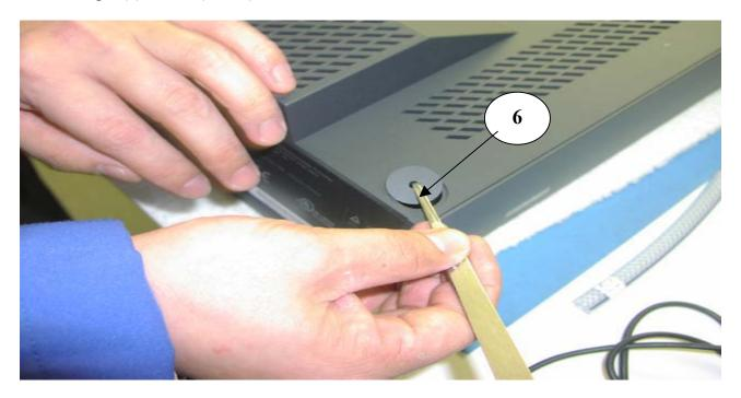
Using tweezers, remove screw covers (Item 6), a total of four (4), one in each corner. Proceed to remove four (4) screws.
