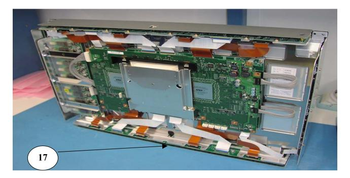
After removing mylar from front polarizer, situate panel assembly (IPN F8991) on edge (Item 17) in preparation for installation into bezel.
