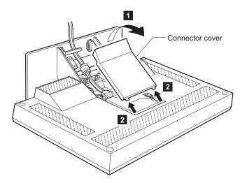
4. Unhook the digital signal cable from the cable hook and lift it up to store the connector tool to the rear compartment of the monitor.
