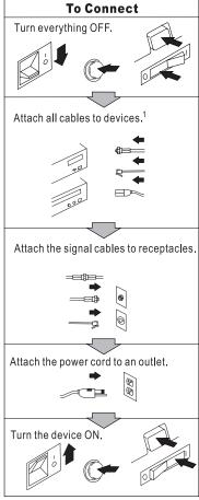
In the U.K., by law, the telephone line cable must be connected after the power cord.
