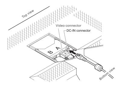
**Note:** The video connectors A and B on the monitor are Safety Extra Low Voltage (SELV) circuits.
