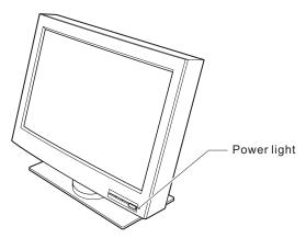
The color of the power light changes from green to amber when your monitor receives a time-out video signal from the computer and enters Standby mode to save power. A time-out video signal is sent from your computer to the monitor when the former detects inactivity on the keyboard or mouse for a set duration of time. You can change the time-out duration for your monitor from the computer. Refer to the manual shipped with your computer to change the time-out duration value.
