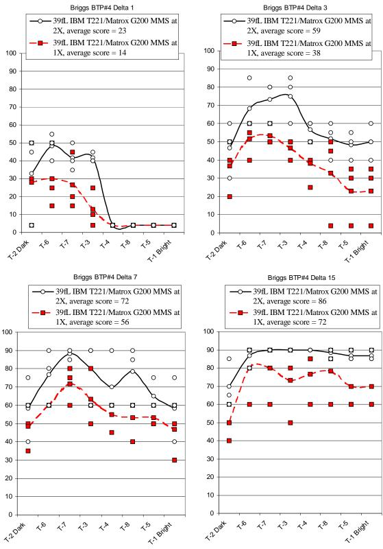
**Figure II.21-6.** Briggs scores for delta-1, delta-3, delta-7, and delta-15 contrast ratios on BPT#4 test pattern for the IBM T221 color LCD with Lmin set to 0.1fL. Lmax was 39 fL. Each of these data points represents an individual score by each of three NIDL observers. The solid line shows the average score for each target, T-1 through T-8.
