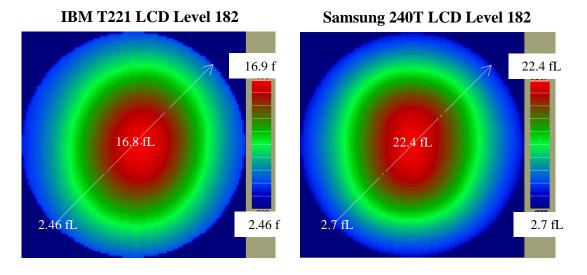
**Figure II.24-8.** Viewing Cone Luminance of gray level 182. The center of the plot is perpendicular to the screen. The edge of the circle is 70 degrees off perpendicular.
