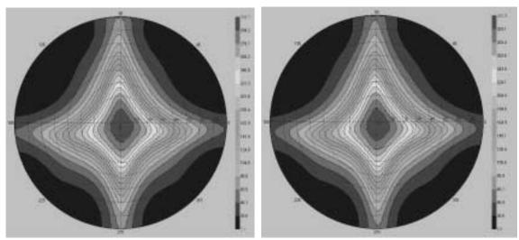
**Figure II.24-14d.** Viewing Cone Luminance of contrast ratio measured by IBM using an ELDIM conoscopic spectrometer. The center of the plot is perpendicular to the screen. The edge of the circle is 80 degrees off perpendicular.
