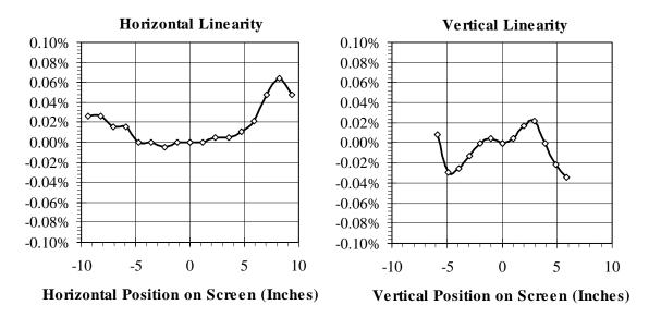
**Fig. II.18-3.** Horizontal and vertical linearity characteristics. The values are well below the 1% maximum needed to pass the IEC requirements.
