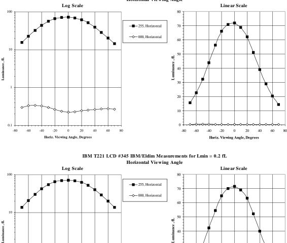
IBM T221 LCD#108 IBM/Eldim Measurements for Lmin = 0.2 fL Horizontal Viewing Angle
