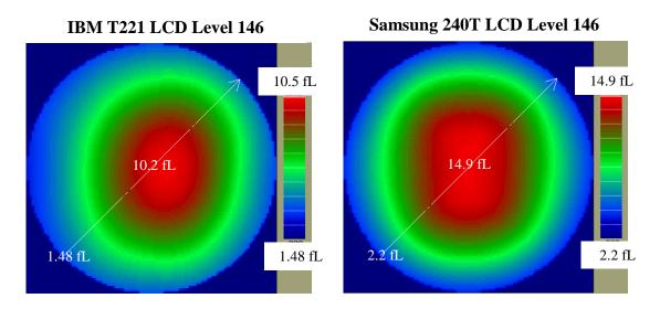
**Figure II.24-9.** Viewing Cone Luminance of gray level 146. The center of the plot is perpendicular to the screen. The edge of the circle is 70 degrees off perpendicular.
