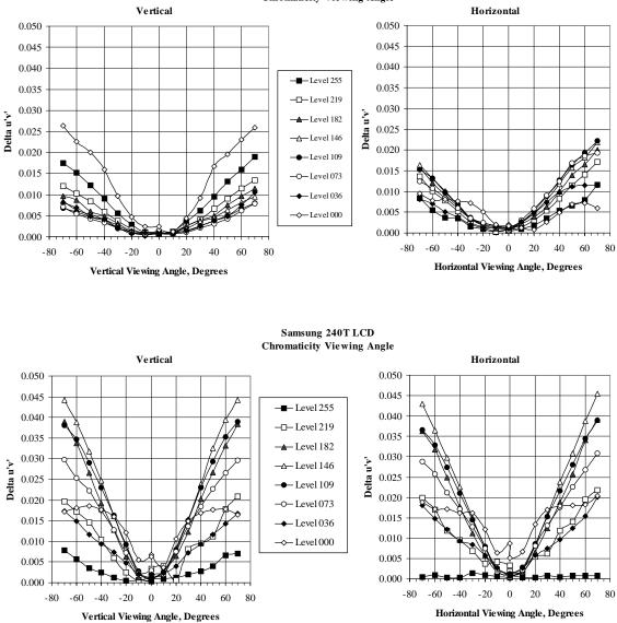
IBM T221 LCD #108 NIDL Measurements for Lmin = 0.1 fL Chromaticity Viewing Angle
