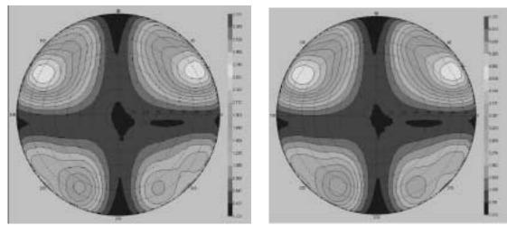
**Figure II.24-14b.** Viewing Cone Luminance of Lmin (level 0) measured by IBM using an ELDIM conoscopic spectrometer. The center of the plot is perpendicular to the screen. The edge of the circle is 80 degrees off perpendicular.
