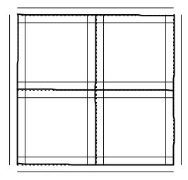
**Figure II.15-3** Waviness of IBM T221 LCD Monitor in 3840 x 2400 mode. Departures from straight lines are exaggerated on a 10X scale. Error bars are +/-0.5% of total screen size. Waviness does not exceed 0.04%.
