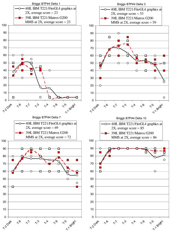
**Figure II.21-5.** Briggs scores for delta-1, delta-3, delta-7, and delta-15 contrast ratios on BPT#4 test pattern for the IBM T221 color LCD with Lmin set to 0.1fL. Lmax was 39 fL. Each of these data points represents an individual score by each of three NIDL observers. The solid line shows the average score for each target, T-1 through T-8.
