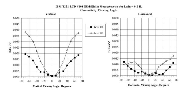
**Figure II.24-5d** Vertical and Horizontal Viewing Angle for Chromaticity of Lmax (white level 255) and Lmin (black level 0) measured by IBM using an ELDIM conoscopic spectrometer for the IBM T221 #108 LCD monitor for Lmin set to 0.2 fL.
