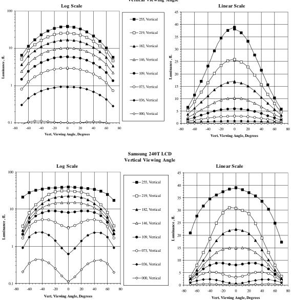
IBM T221 LCD #108 NIDL Measurements for Lmin = 0.1 fL Vertical Viewing Angle
