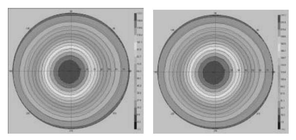
**Figure II.24-14a.** Viewing Cone Luminance of Lmax (level 255). The center of the plot is perpendicular to the screen. The edge of the circle is 80 degrees off perpendicular.
