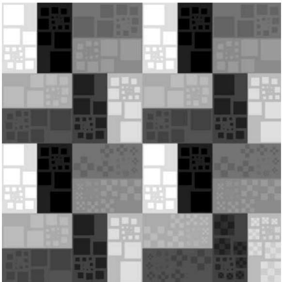
**Figure II.21-2.** 1024 x 1024 mosaic comprised of four 512 x 512 Briggs BPT#4 Test Patterns. The upper left quadrant contains the set of 8 Briggs targets with command contrast of delta 1. The upper right quadrant contains command contrast of delta 3. Delta 7 targets are in the lower left quadrant and delta 15 targets are in the lower right.
