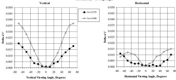
**Figure II.24-5b** Vertical and Horizontal Viewing Angle for Chromaticity of Lmax (white level 255) and Lmin (black level 0) measured by NIDL using a Microvision goniometric spectrometer, and measured by IBM using an ELDIM conoscopic spectrometer for the IBM T221 #108 LCD monitor for Lmin set to 0.1 fL.
