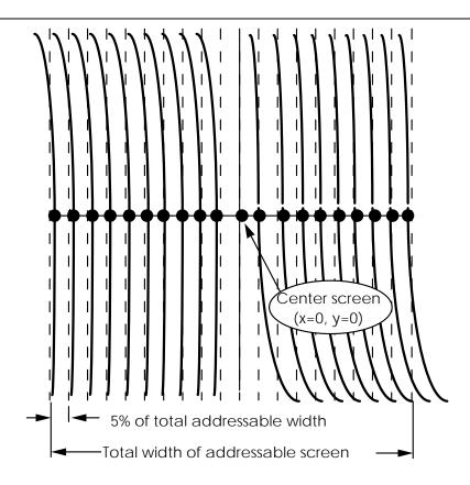
**Figure II.18-2.** Measurement locations for horizontal linearity along the major axis of the display. Equal pixel spacings between vertical lines in the grille pattern are indicated by the dotted lines. The number of pixels per space is nominally equivalent to 5% of the addressable screen size.
