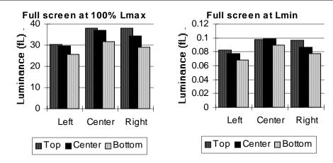
**Figure II.3-3.** 9-Point (3 x 3 grid) Sampled Spatial Uniformity of Luminance (Lmax and Lmin).
