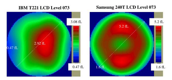
**Figure II.24-11.** Viewing Cone Luminance of gray level 073. The center of the plot is perpendicular to the screen. The edge of the circle is 70 degrees off perpendicular.
