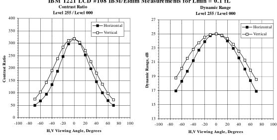
IBM T221 LCD #108 IBM/Eldim Measurements for Lmin = 0.1 fL
