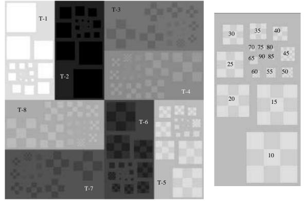
**Figure II.21.1.** Briggs BPT#4 Test Patterns comprised of 8 targets labeled T-1 through T-8. A series of 17 checkerboards is contained within each of the 8 targets. Each checkerboard is assigned a score value ranging from 10 to 90. Higher scores are assigned to smaller checkerboards.
