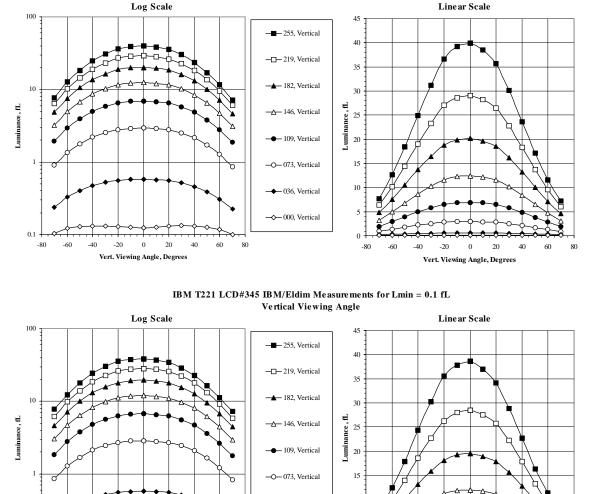
IBM T221 LCD #108 IBM/Eldim Measurements for Lmin = 0.1 fL Vertical Viewing Angle
