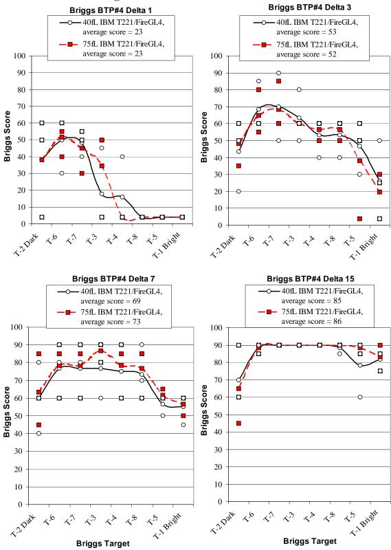
**Figure II.21-4.** Briggs scores for delta-1, delta-3, delta-7, and delta-15 contrast ratios on BPT#4 test pattern for the IBM T221 color LCD with Lmax set to 40 fL and to 75 fL. Each of these data points represents an individual score by each of three NIDL observers. The solid line shows the average score for each target, T-1 through T-8.
