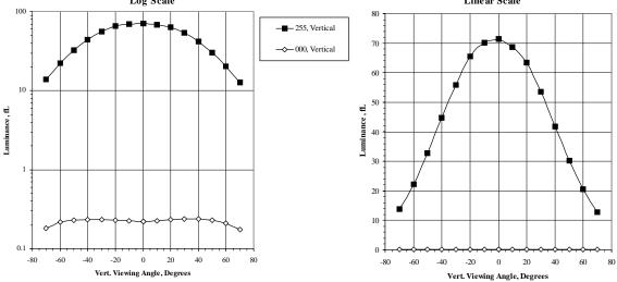
**Figure II.24-3c.** Vertical Viewing Angle for Lmax (level 255) and Lmin (level 0) measured by IBM using an ELDIM conoscopic spectrometer for the IBM T221 #108 LCD compared to the IBM T221 #345 LCD monitor for Lmin set to 0.2 fL. For both the IBM T221 LCDs, the data shows a 50% drop in luminance when viewed 45 degrees from the perpendicular. The 50% drop in luminance occurs at level 255.
