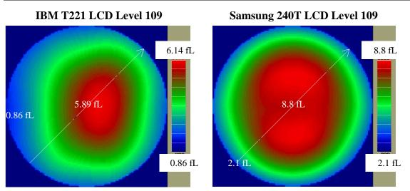
**Figure II.24-10.** Viewing Cone Luminance of gray level 109. The center of the plot is perpendicular to the screen. The edge of the circle is 70 degrees off perpendicular.
