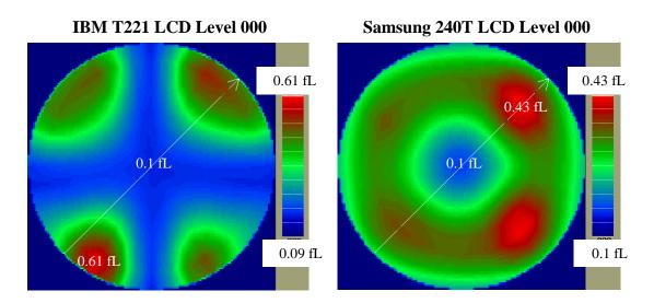
**Figure II.24-13.** Viewing Cone Luminance of Lmin (level 000). The center of the plot is perpendicular to the screen. The edge of the circle is 70 degrees off perpendicular.
