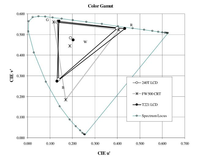
Figure II.25.1. CIE chromaticity coordinates and color gamut of the IBM T221 LCD monitor compared to the Samsung 240T LCD monitor and the Sony FW500 color CRT monitor.
