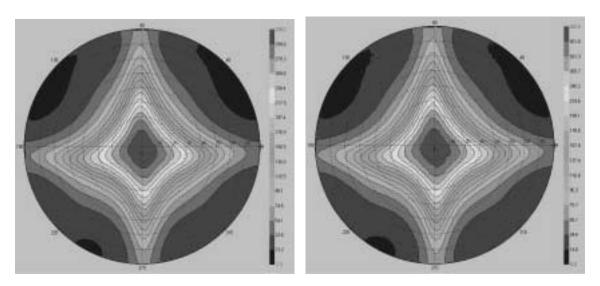
**Figure II.24-14c.** Viewing Cone Luminance of contrast ratio measured by IBM using an ELDIM conoscopic spectrometer. The center of the plot is perpendicular to the screen. The edge of the circle is 80 degrees off perpendicular.
