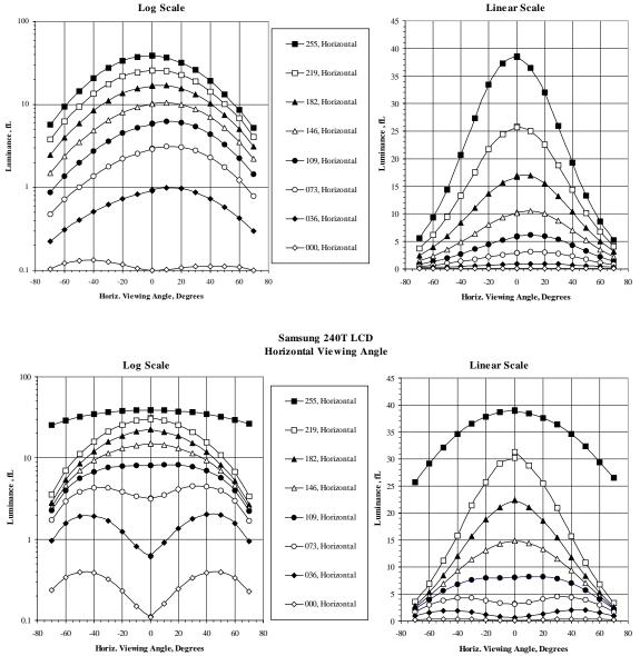
IBM T221 LCD #108 NIDL Measurements for Lmin = 0.1 fL Horizontal Viewing Angle
