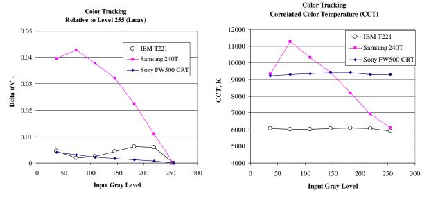
**Figure II.5-2.** Chromaticity and color temperature shift of measured white points for gray levels shown relative to Lmax (Level 255) for the IBM T221 LCD monitor compared to the Samsung 240T LCD and Sony FW900 CRT monitors. The T221 has excellent color tracking.
