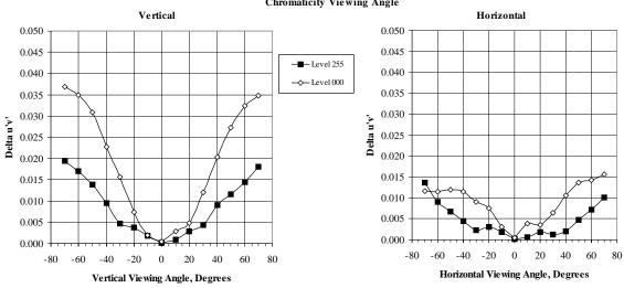
IBM T221 LCD#345 IBM/Eldim Measurements for Lmin = 0.1 fL Chromaticity Viewing Angle
