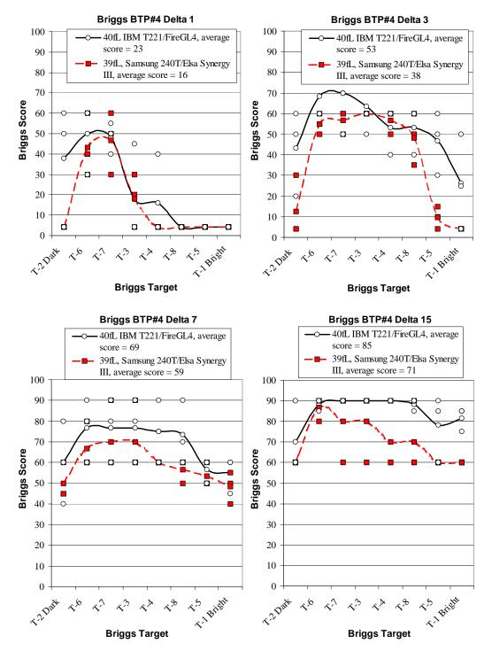
**Figure II.21-3.** Briggs scores for delta-1, delta-3, delta-7, and delta-15 contrast ratios on BPT#4 test pattern for the IBM T221 color LCD compared to Samsung 240T color LCD monitor. Each of these data points represents an individual score by each of three NIDL observers. The solid line shows the average score for each target, T-1 through T-8.
