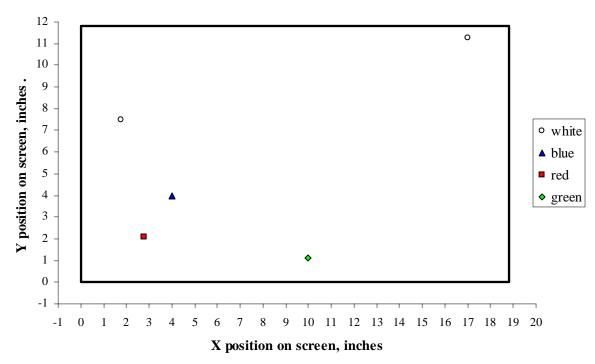
Figure II.22-1. Locations of pixel deflects observed on the IBM T221 LCD monitor.
