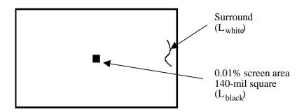
Figure II.4-1 Test pattern for measuring halation.
