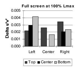
**Figure II.3-4.** 9-Point (3 x 3 grid) Sampled Spatial Uniformity of White (Lmax) Chromaticity. (Delta u'v' of 0.004 is just visible.)
