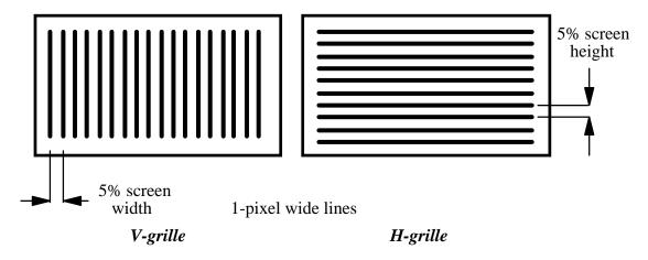
Figure II.18-1. Grille patterns for measuring linearity
