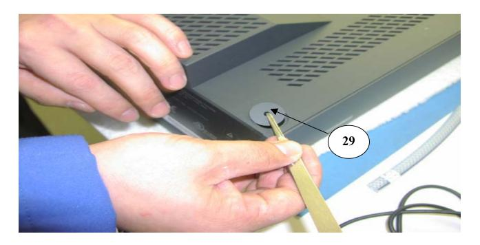
Insert four (4) screws into the rear cover, one in each corner. Replace screw covers (Item 29).
