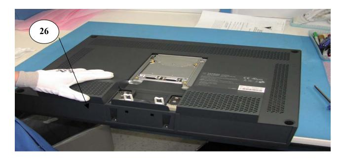
Place back cover (Item 26) onto panel assembly, ensuring cover is fully seated.
