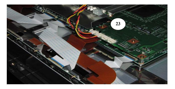
Ensure both fan cables are securely seated and in their original connector positions (Item 23).
