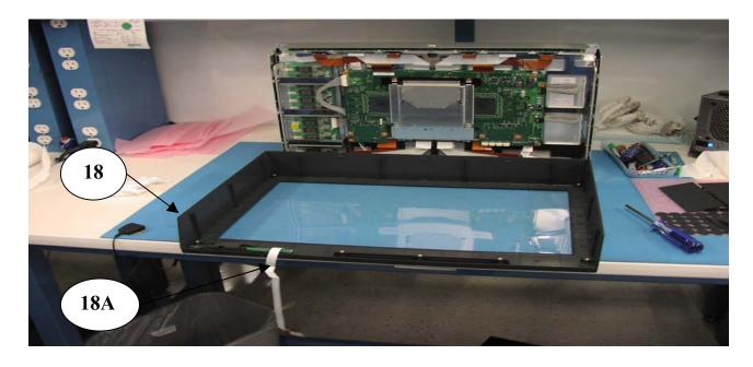
Situate bezel (Item 18) in front of panel. Place the bottom of bezel (with cable- Item 18A) off the table edge to protect the underlying function control buttons.
