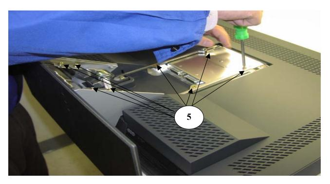
Remove eight (8) screws (Item 5) that secure monitor base. Lift and remove base from monitor.
