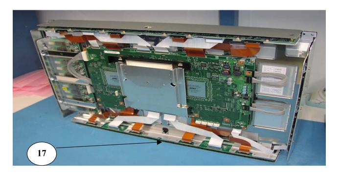
After removing mylar from front polarizer, situate panel assembly (IPN F8991) on edge (Item 17) in preparation for installation into bezel.
