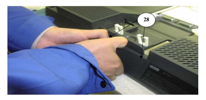
Grasp and install cover panel (Item 28) by snapping into position.
