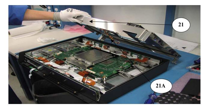
Situate metal backbone (Item 21) over panel and lower onto panel, enough to connect the two (2) fan cables (Item 21A).
