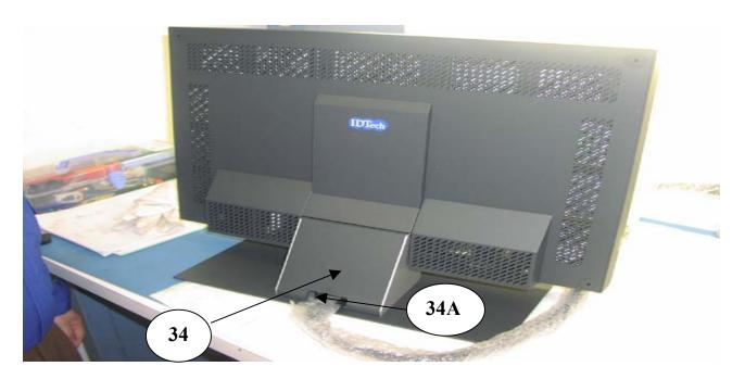
Install lower rear cover panel (Item 34) by snapping into position. Ensure interface cables routed through the opening (Item 34A). Monitor assembly is complete.
