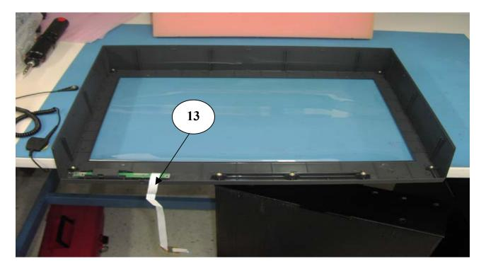
Lay bezel on bench to inspect for any damage; pay particular attention to function cable (Item 13).
