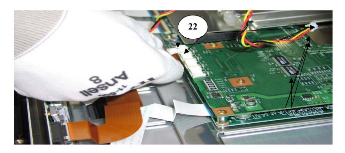
Connect two (2) fan cables into the original connector mates on the PCB (Item 22). Do not mix.
