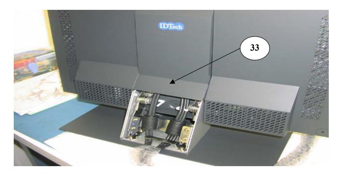
Install upper rear cover panel (Item 33) by snapping into position.
