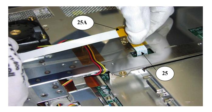
Insert control cable into connector (Item 25) and restick tape (Item 25A).
