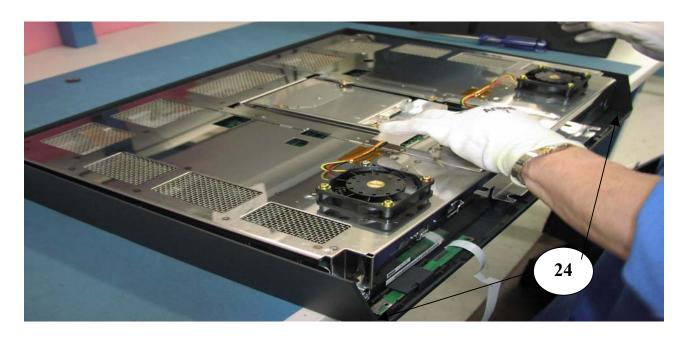
Lower backbone fully into the bezel, ensuring backbone is properly seated (Item 24).
