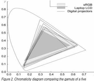
Figure 2. Chromaticity diagram comparing the gamuts of a five different digital projectors to the sRGB display gamut and that of a typical laptop LCD display.
