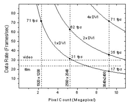
Figure 1. Data frame-rate limitations of DVI channels providing 165Mpixel/sec.
