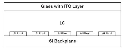
Figure 1. Schematic of the basic structure of an LCoS microdisplay.
