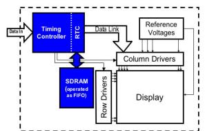
Figure 3. An example of RTC overdrive in the system. Highlighted is the added function of the timing controller in the LCD module. An external RAM is used as frame FIFO (first in, first out) memory.
