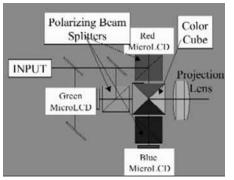
Figure 3. Typical three-color projection optical system for LCoS.
